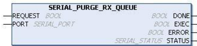
Figure 158: Block Used to Clean the RX Queue
