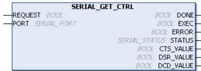
Figure 105: Block Used to Visualize the Control Signals
