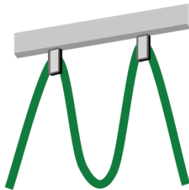
Figure 3-25. Trailing and festoon cables
