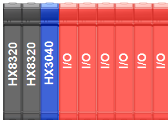
Figure 1: Power Supply Redundancy
