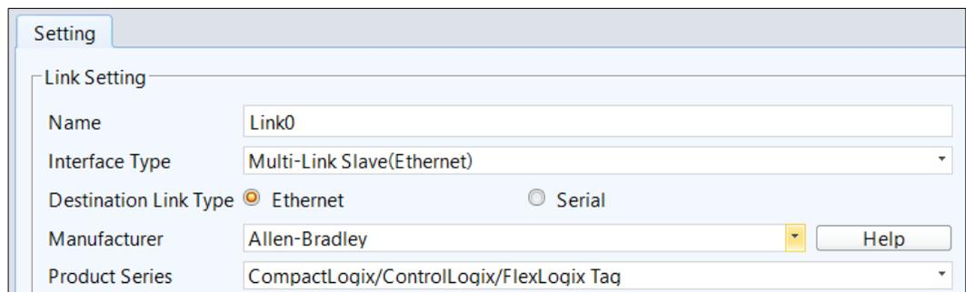
The screenshot shows the 'Setting' dialog box with the 'Link Setting' section expanded. The fields are: Name: Link0; Interface Type: Multi-Link Slave(Ethernet); Destination Link Type: Ethernet (selected); Manufacturer: Allen-Bradley; Product Series: CompactLogix/ControlLogix/FlexLogix Tag. There is a 'Help' button next to the Manufacturer field.
