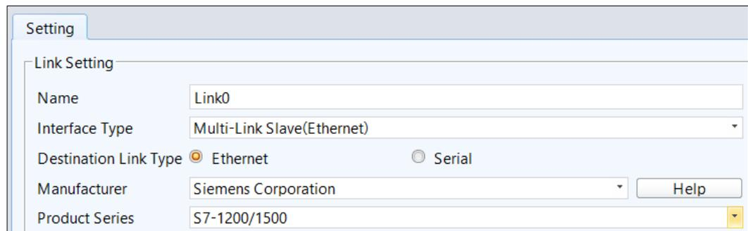
The screenshot shows the 'Setting' dialog box with the 'Link Setting' section expanded. The fields are: Name: Link0; Interface Type: Multi-Link Slave(Ethernet); Destination Link Type: Ethernet (selected); Manufacturer: Siemens Corporation; Product Series: S7-1200/1500. There is a 'Help' button next to the Manufacturer field.
